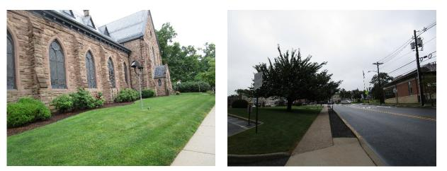
A rain garden can be installed in the turfgrass along the side of the church to capture, treat, and infiltrate stormwater runoff from the roof. An existing asphalt strip adjacent to the sidewalk can be replaced with a series of stormwater planters that could capture stormwater from the roadway. A preliminary soil assessment suggests that more soil testing would be required before determining the soil's suitability for green infrastructure.
