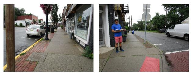
A stormwater planter can be installed near the catch basin to intercept stormwater coming from the roadway. A tree filter box can be installed in the sidewalk area to capture additional runoff from the roadway. A preliminary soil assessment suggests that more soil testing would be required before determining the soil's suitability for green infrastructure.
