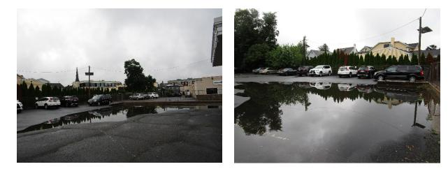
Parking spaces in the parking lot at the back of the building can be converted to porous pavement to capture and infiltrate stormwater runoff from the parking lot. Porous pavement can also help drain the large pooling area of the parking lot. A preliminary soil assessment suggests that the soils have suitable drainage characteristics for green infrastructure.
