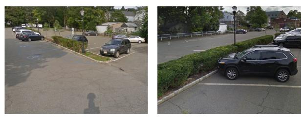
Parking spaces throughout the lot can be converted to porous pavement to capture and infiltrate stormwater runoff from the rest of the parking lot. A preliminary soil assessment suggests that more soil testing would be required before determining the soil's suitability for green infrastructure.
