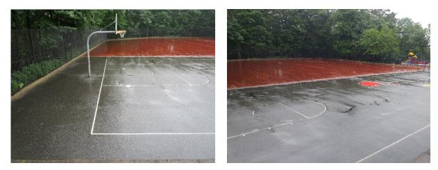
Porous pavement can be installed at the back of the building in the playground to capture runoff from the large area of pavement. A preliminary soil assessment suggests that more soil testing would be required before determining the soil's suitability for green infrastructure.
