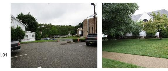
Parking spaces can be converted to porous pavement to capture and infiltrate stormwater runoff from the parking lot. Rain gardens can be installed in the turfgrass areas at the eastern side of the building to capture, treat, and infiltrate stormwater runoff from the roof if the downspouts are disconnected. A preliminary soil assessment suggests that the soils have suitable drainage characteristics for green infrastructure.
