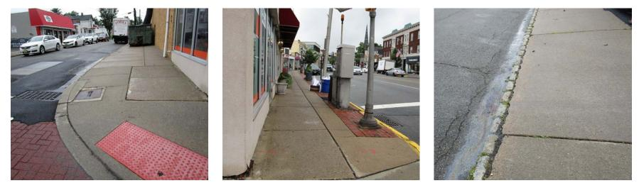
Stormwater planters can be installed in the sidewalk area before the catch basin to intercept stormwater coming from the roadway. A tree filter box can also be installed in the sidewalk area to filter additional runoff from the roadway. A preliminary soil assessment suggests that more soil testing would be required before determining the soil's suitability for green infrastructure.
