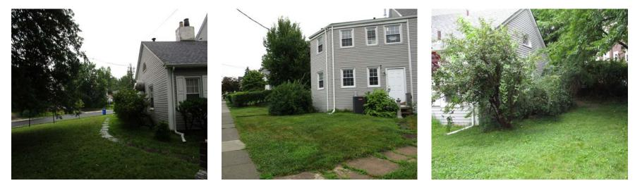
A rain garden can be installed in the turfgrass area near the downspouts of the southeast corner near the entrance of the building to capture, treat, and infiltrate stormwater runoff from the roof. Two other rain gardens can be installed along the west end of the building by redirecting downspouts into the gardens. A preliminary soil assessment suggests that more soil testing would be required before determining the soil's suitability for green infrastructure.
