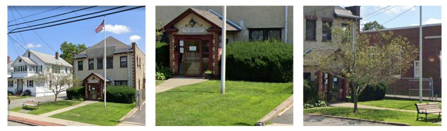
A rain garden can be installed at the front of the building around the flag pole by disconnecting the downspout from the corner of the building into the garden. A preliminary soil assessment suggests that the soils have suitable drainage characteristics for green infrastructure.
