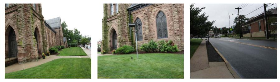
A rain garden can be installed in the turfgrass along the side of the church to capture, treat, and infiltrate stormwater runoff from the roof. An existing asphalt strip adjacent to the sidewalk can be replaced with a series of stormwater planters that could capture stormwater from the roadway. A preliminary soil assessment suggests that more soil testing would be required before determining the soil's suitability for green infrastructure.
