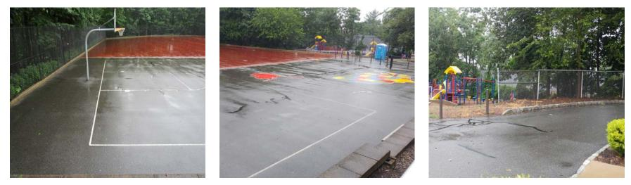
Porous pavement can be installed at the back of the building in the playground to capture runoff from the large area of pavement. A preliminary soil assessment suggests that more soil testing would be required before determining the soil's suitability for green infrastructure.
