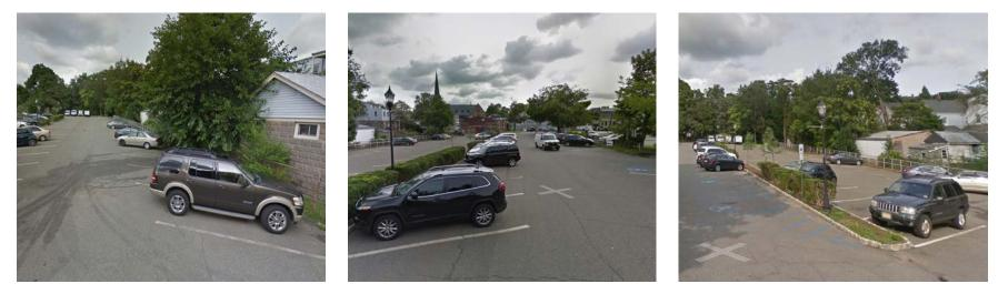
Parking spaces throughout the lot can be converted to porous pavement to capture and infiltrate stormwater runoff from the rest of the parking lot. A preliminary soil assessment suggests that more soil testing would be required before determining the soil's suitability for green infrastructure.
