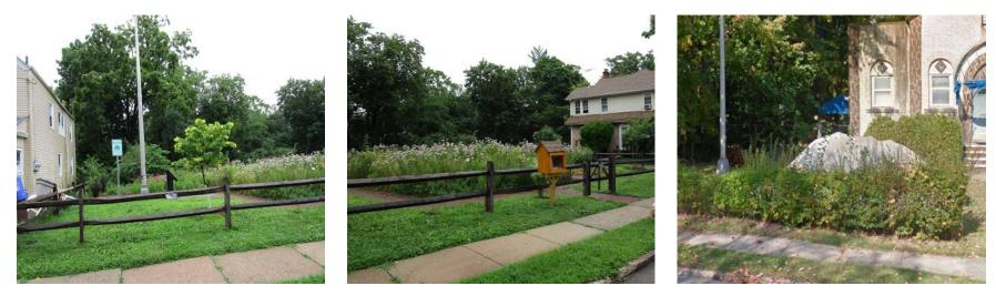
A rain garden can be installed in the turfgrass area along the fence to capture, treat, and infiltrate stormwater runoff from the roadway. A preliminary soil assessment suggests that the soils have suitable drainage characteristics for green infrastructure.
