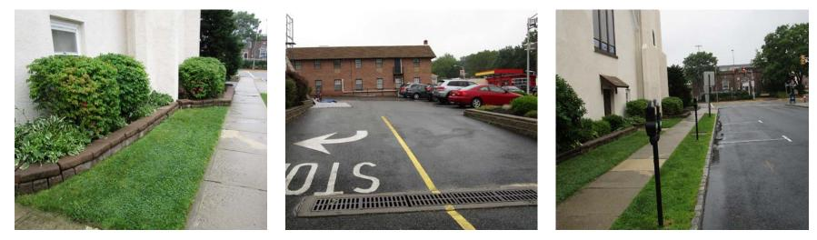
A rain garden can be installed in the turfgrass and shrub area along the side of the building to capture, treat, and infiltrate stormwater runoff from the roof. Parking spaces in the parking lot can be converted to porous pavement to capture and infiltrate stormwater runoff from the front parking lot. A preliminary soil assessment suggests that more soil testing would be required before determining the soil's suitability for green infrastructure.
