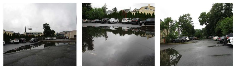
Parking spaces in the parking lot at the back of the building can be converted to porous pavement to capture and infiltrate stormwater runoff from the parking lot. Porous pavement can also help drain the large pooling area of the parking lot. A preliminary soil assessment suggests that the soils have suitable drainage characteristics for green infrastructure.
