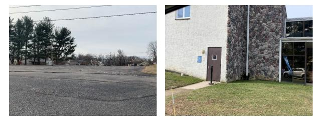
Rain gardens can be placed around the building to capture, treat, and infiltrate the stormwater runoff from the building rooftop. Sections of parking spaces can be converted to pervious pavement to capture the stormwater runoff from the parking lot. A preliminary soil assessment suggests that the soils have suitable drainage characteristics for green infrastructure.
