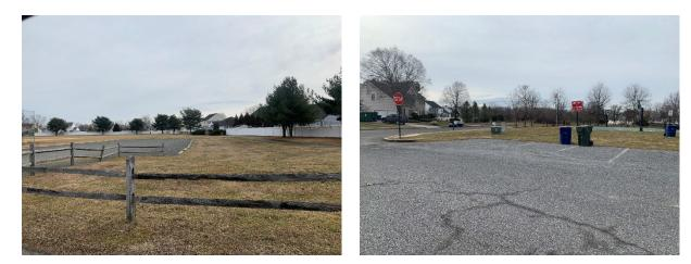
Parking spaces in the south parking lot can be converted to porous pavement to capture and infiltrate stormwater runoff from the parking lot. Rain gardens can be installed alongside the pavement to capture, treat, and infiltrate the stormwater runoff from the parking. A bioswale can be installed alongside the eastern parking lot to help move the stormwater off the parking area. A preliminary soil assessment suggests that the soils have suitable drainage characteristics for green infrastructure.
