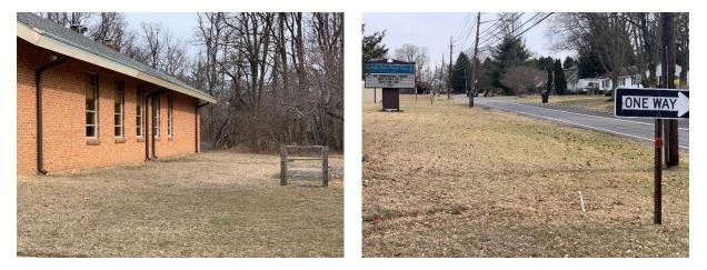
A rain garden can be installed south of the building to capture, treat, and infiltrate the stormwater from three of the downspouts. A bioswale can be installed near the right of way on the street to help prevent erosion of the pavement edge of the street. A preliminary soil assessment suggests that the soils have suitable drainage characteristics for green infrastructure.
