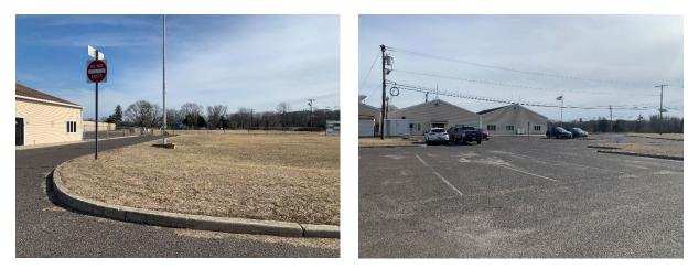
Rain gardens can be installed south of the building and pavement sections to capture, treat, and infiltrate the stormwater runoff from the buildings and roadways. The center of the parking lot can be converted to pervious pavement to promote stormwater infiltration. A preliminary soil assessment suggests that more soil testing would be required before determining the soil's suitability for green infrastructure.
