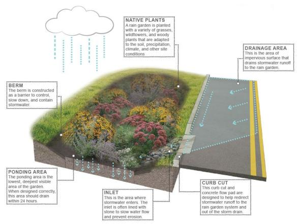
Figure 1: Bioretention system/rain garden
