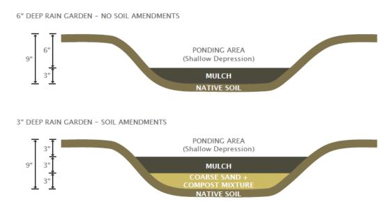
Figure 2: Standard cross-sections of rain gardens
