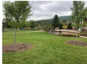
Two rain gardens can be installed northwest of the entrance of the building to capture, treat, and infiltrate stormwater runoff from the patio area. A preliminary soil assessment suggests that the soils have suitable drainage characteristics for green infrastructure.
