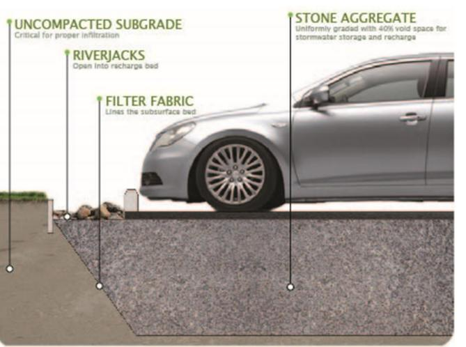
PERMEABLE PAVEMENT DIAGRAM
