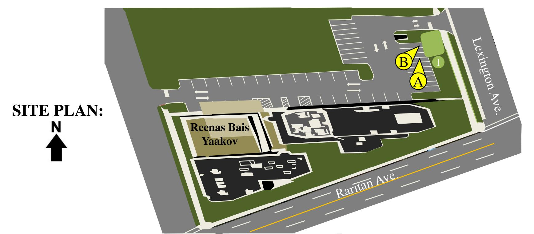
1 BIORETENTION SYSTEMS: A bioretention system could be installed on the turf grass area parallel to Lexington Avenue.
