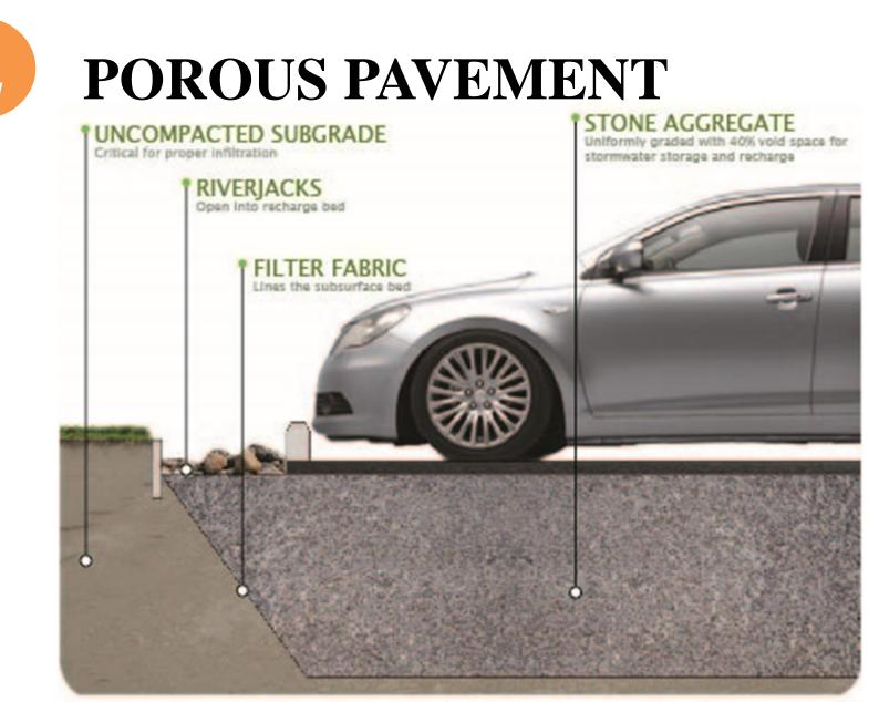
PERMEABLE PAVEMENT DIAGRAM
