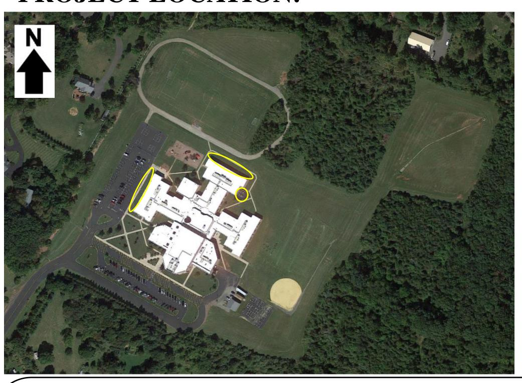
**BIORETENTION SYSTEM:** Bioretention systems could be installed along the sides of the school after disconnecting several downspouts. Bioretention systems will reduce runoff and allow stormwater infiltration, decreasing the amount of contaminants reaching catch basins.
