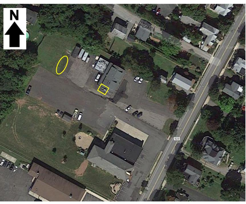
**BIORETENTION SYSTEM:** A bioretention system could be installed in the grass area towards the back of the parking lot to manage stormwater runoff from the parking lot. A bioretention system will reduce runoff and allow stormwater infiltration, decreasing the amount of contaminants reaching catch basins.
