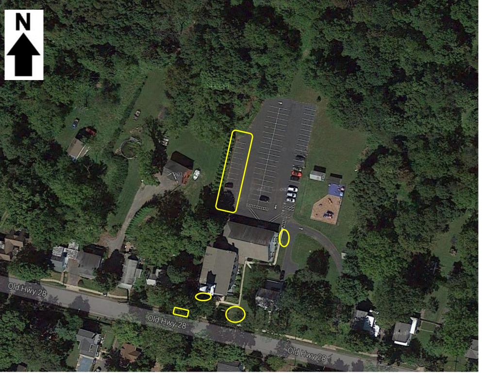
BIORETENTION SYSTEM: Bioretention systems could be installed near the entrance of the building to intercept runoff from downspouts. A bioretention system could also be installed near the eastern side of the rear building to capture runoff from a downspout. A bioretention system will reduce runoff and allow stormwater infiltration, decreasing the amount of contaminants reaching catch basins.
