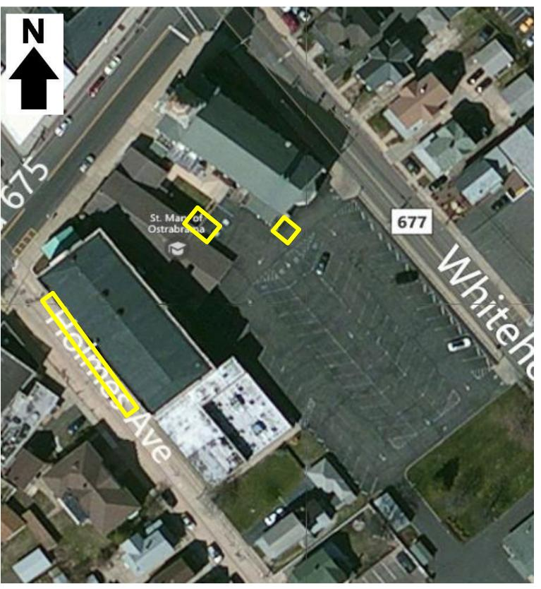
**POROUS PAVEMENT:** Porous pavement can be installed on the sidewalk along Holmes Avenue to collect roof runoff from existing disconnected downspouts. Porous pavement promotes groundwater recharge and filters stormwater.
