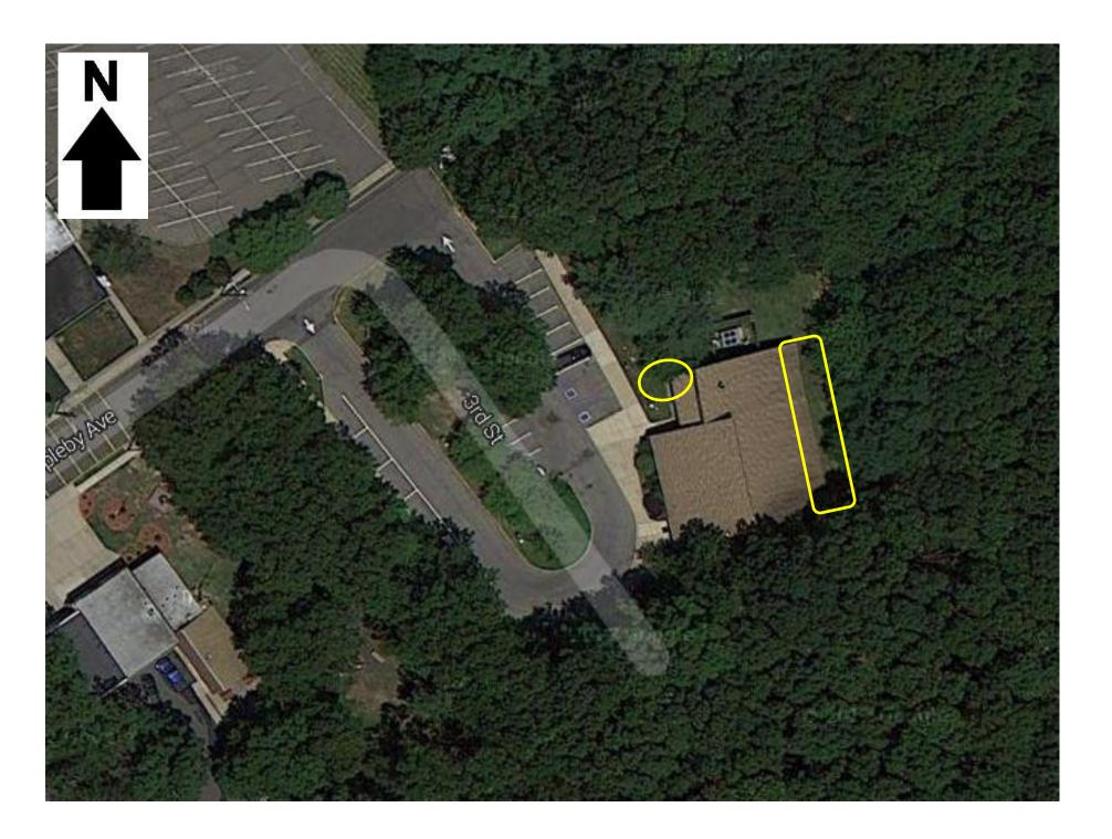
**BIORETENTION SYSTEM:** Bioretention systems could be installed at the northern corner and along the eastern side of the library. A bioretention system will reduce runoff and allow stormwater infiltration, decreasing the amount of contaminants that reaches catch basins.
