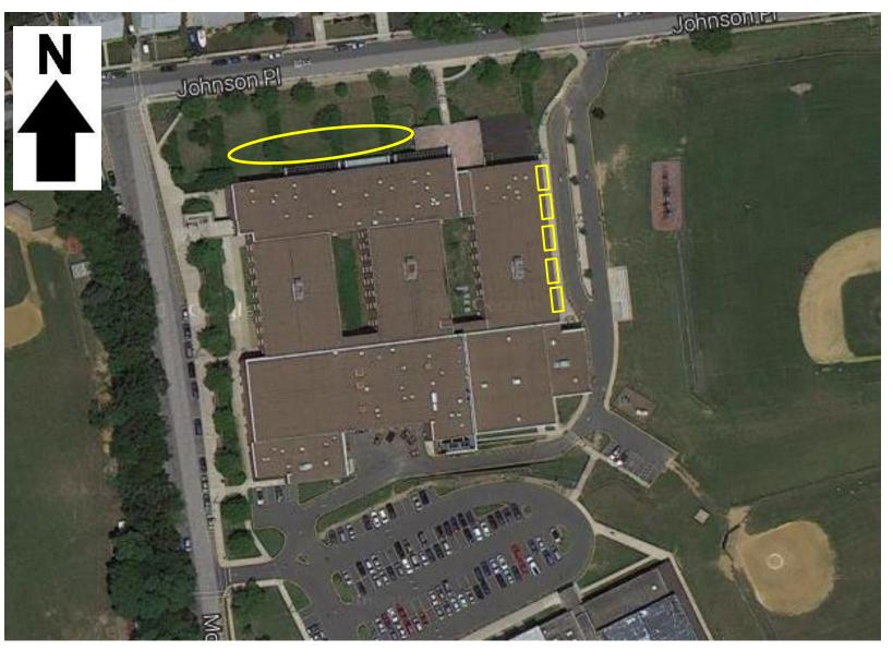
**BIORETENTION SYSTEM:** A bioretention system could be installed along the northern side of the building after disconnecting downspouts. A bioretention system will reduce runoff and allow stormwater infiltration, decreasing the amount of contaminants that reaches catch basins.
