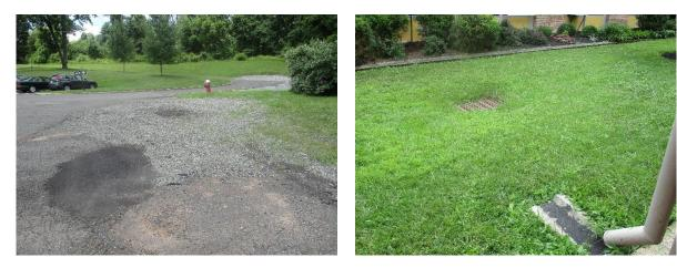
On the west side of the building, a downspout flows directly into a catch basin. A rain garden can be installed before the catch basin to intercept and treat the rooftop runoff. A preliminary soil assessment suggests that more soil testing would be required before determining the soil's suitability for green infrastructure.
