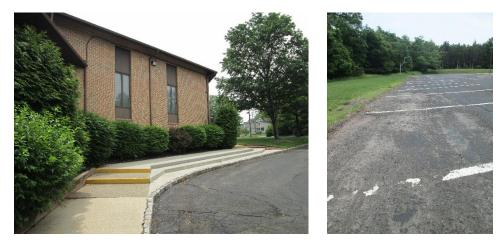
The northern parking lot drains to one catch basin in the northeast area of the site. A rain garden can be installed adjacent to the catch basin to capture, treat, and infiltrate stormwater runoff. A preliminary soil assessment suggests that the soils have suitable drainage characteristics for green infrastructure.
