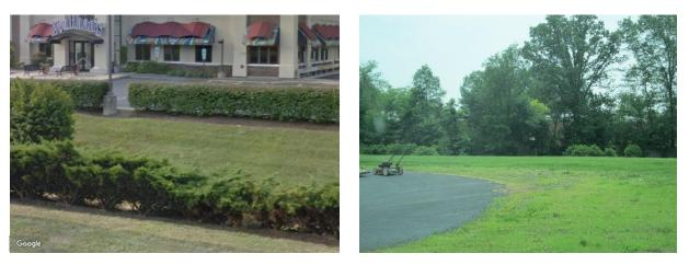
In the back parking lot there is evidence of erosion in the turf grass. A bioretention system can be installed in this area along the curve of the driveway to capture, treat, and infiltrate stormwater runoff. A preliminary soil assessment suggests that more soil testing would be required before determining the soil's suitability for green infrastructure.
