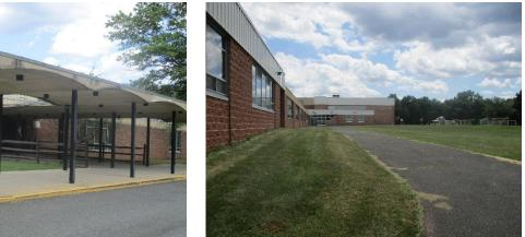
A rain garden can be installed on the east side of the school to mange runoff from the driveway. An area of eroded pavement can also be converted into pervious pavement to infiltrate stormwater. A preliminary soil assessment suggests that the soils have suitable drainage characteristics for green infrastructure.
