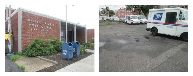
The mail truck parking area has some pooling and erosion concerns and runoff currently flows into the road. Pervious pavement can be used to capture and infiltrate this runoff. The building has internal drainage. A preliminary soil assessment for this site suggests that soils have suitable drainage characteristics for green infrastructure.
