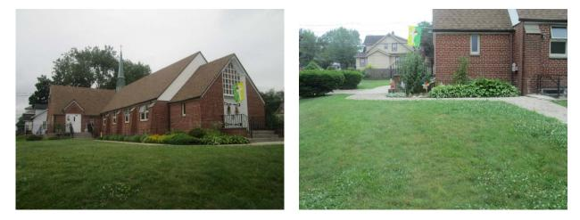
Two bioretention systems can be implemented on either side of the main entrance. A rain barrel can be used to water both existing and proposed gardens. The paved driveway can also be redone with pervious pavement. A preliminary soil assessment for this site suggests that soils have suitable drainage characteristics for green infrastructure.
