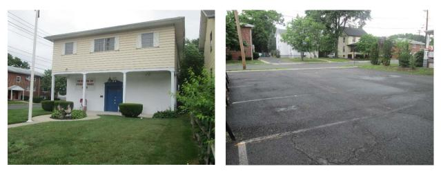
Parking lot runoff currently flows toward the street. The parking lot can be partially redone with pervious pavement to capture this runoff as well as some of the roof runoff. The building has disconnected downspouts, which can also be directed into two bioretention systems in order to capture, treat and infiltrate runoff. A preliminary soil assessment for this site suggests that soils have suitable drainage characteristics for green infrastructure.
