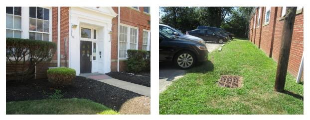
Parking spaces can be replaced with pervious pavement to capture and infiltrate stormwater. Bioretention systems can also be installed to capture, treat, and infiltrate runoff. A preliminary soil assessment suggests that the soils have suitable drainage characteristics for green infrastructure.
