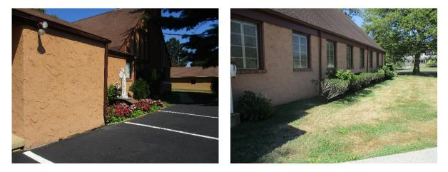
Parking spaces can be replaced with porous asphalt to capture and infiltrate stormwater. Installing rain gardens adjacent to the building can capture, treat, infiltrate roof runoff. A preliminary soil assessment suggests that the soils have suitable drainage characteristics for green infrastructure.
