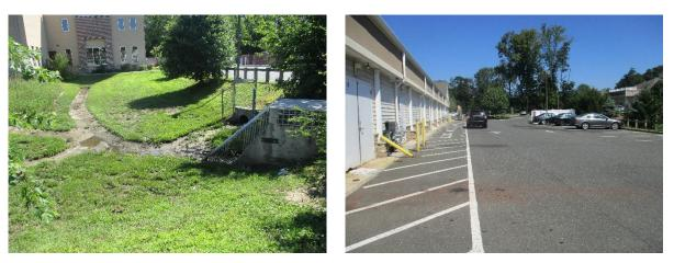
Parking spaces can be replaced with porous asphalt to capture and infiltrate runoff. A preliminary soil assessment suggests that the soils have suitable drainage characteristics for green infrastructure.
