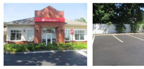
Parking spaces can be replaced with porous asphalt to capture and infiltrate stormwater. A preliminary soil assessment suggests that the soils have suitable drainage characteristics for green infrastructure.
