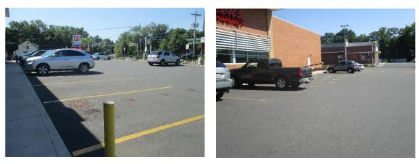
Parking spaces can be replaced with porous asphalt to capture and infiltrate stormwater runoff. A preliminary soil assessment suggests that the soils have suitable drainage characteristics for green infrastructure.
