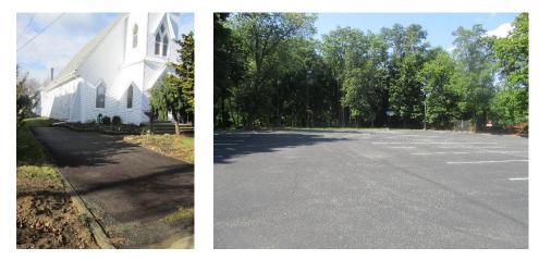
Parking spots west of the building can be replaced with porous asphalt to capture and infiltrate stormwater runoff. A preliminary soil assessment suggests that the soils have suitable drainage characteristics for green infrastructure.
