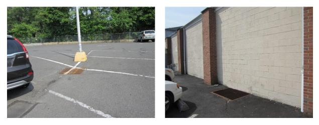
Parking spaces can be replaced with porous asphalt to infiltrate stormwater. A rain garden can also be installed in the turf grass island south of the store to capture, treat and infiltrate parking lot runoff. A preliminary soil assessment suggests that more soil testing would be required before determining the soil's suitability for green infrastructure.
