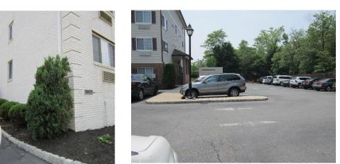
Parking spaces can be repaved with porous asphalt to reduce impervious cover and infiltrate stormwater. A downspout at the east corner of the building can also be disconnected into a cistern to harvest rainwater that the residents can use for watering the existing plants. A preliminary soil assessment suggests that more soil testing would be required before determining the soil's suitability for green infrastructure.
