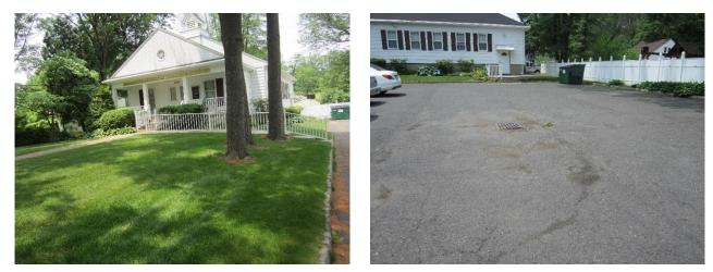
Parking spaces can be replaced with pervious pavement to infiltrate runoff. A rain garden can also capture, treat and infiltrate stormwater. A preliminary soil assessment suggests that more soil testing would be required before determining the soil's suitability for green infrastructure.
