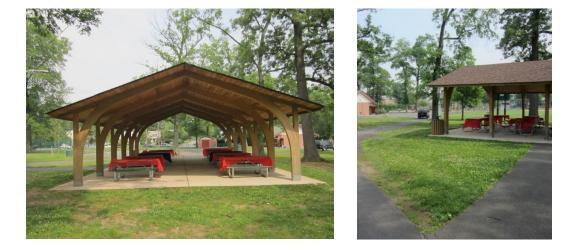
Gutters and downspouts can be installed on the pavilion at the center of the park. A bioretention system can then be installed in the adjacent turf grass to capture, treat, and infiltrate runoff from the roof. A preliminary soil assessment suggests that the soils have suitable drainage characteristics for green infrastructure.
