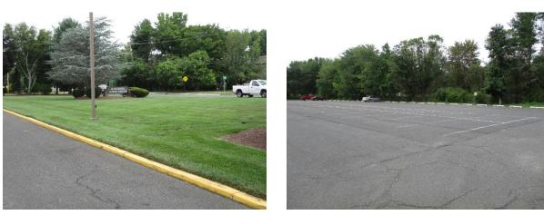
Most of the building has internal drainage. The front driveway drains into the roadway, and the parking lot drains into a swale near the highway. A rain garden can be installed in front of the building to treat stormwater from the driveway. Pervious pavement can replace parking spaces along the southwest edge of the parking lot to capture and infiltrate runoff. A preliminary soil assessment suggests that the soils have suitable drainage characteristics for green infrastructure.
