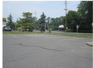
Stormwater from the roof flows through disconnected downspouts onto the pavement. Rain gardens can be constructed at two locations to capture, treat, and infiltrate parking lot runoff. Parking spaces can also be replaced with pervious pavement to capture and infiltrate additional stormwater. A preliminary soil assessment suggests that the soils have suitable drainage characteristics for green infrastructure.
