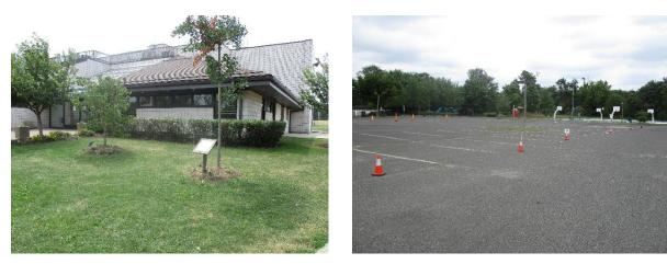
The recreation center's parking lot drains to the north. Parking spaces can be converted into pervious pavement to capture and infiltrate this runoff. The building already has disconnected downspouts that flow onto the grass and then into catch basins. Rain gardens can be installed to capture, treat and infiltrate this runoff. A preliminary soil assessment suggests that the soils have suitable drainage characteristics for green infrastructure.
