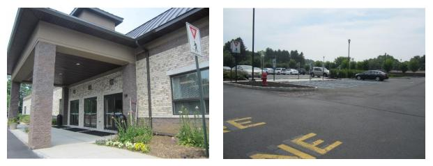
Runoff from the roof and parking lot appears to drain into an existing bioswale. A rain garden can be constructed in the turf grass area south of the Worship Center to capture, treat, and infiltrate some of this runoff. A preliminary soil assessment suggests that more soil testing would be required before determining the soil's suitability for green infrastructure.
