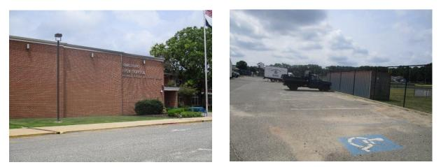
Most of the building has internal drainage, except at the front where downspouts drain onto the driveway. A rain garden can be constructed in front of the school to capture, treat, and infiltrate runoff. Pervious pavement can also be used to replace parking spaces to capture and infiltrate stormwater runoff. A preliminary soil assessment suggests that the soils have suitable drainage characteristics for green infrastructure.
