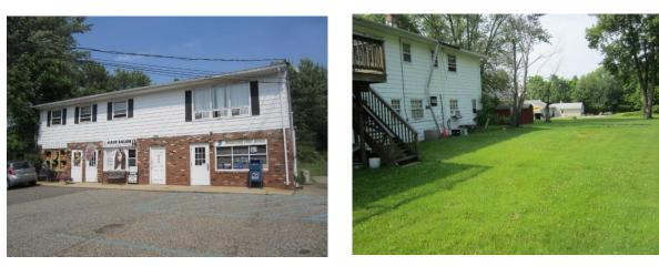
Roof runoff flows through disconnected downspouts into the parking lot, and to the rear of building. Parking spaces can be replaced with pervious pavement to capture parking lot and roof runoff. A rain garden can installed in the rear of the building to capture, treat, and infiltrate roof runoff as well. A preliminary soil assessment suggests that more soil testing would be required before determining the soil's suitability for green infrastructure.
