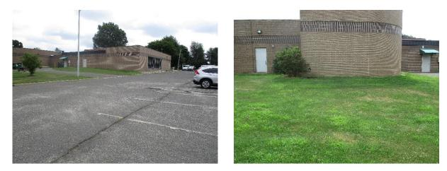
This library's parking lot drains into a turf grass field. Rain gardens can capture, treat, and infiltrate this runoff, as well as some of the buildings rooftop runoff. A preliminary soil assessment suggests that the soils have suitable drainage characteristics for green infrastructure.
