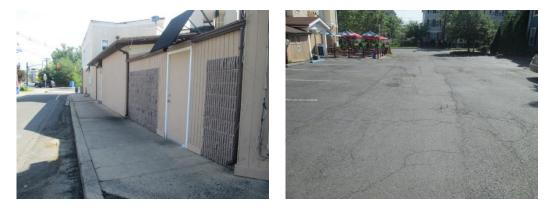
The parking lot drains to the roadway. Parking spaces can be replaced with porous asphalt to infiltrate stormwater. Pervious concrete can be installed to capture roof runoff draining onto the sidewalk on the west side of the building. A preliminary soil assessment suggests that the existing soils have suitable drainage characteristics for green infrastructure.
