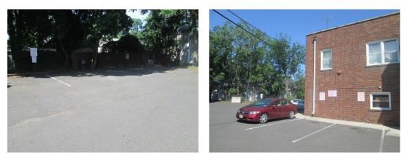
The rear of the shopping complex has a parking area which drains toward the street. Porous asphalt can be installed in the spaces along the building to infiltrate stormwater and capture roof runoff from the disconnected downspout. A preliminary soil assessment suggests that the existing soils have suitable drainage characteristics for green infrastructure.
