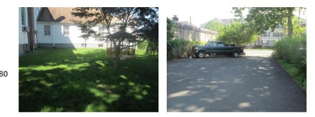
A rain garden can be installed to capture roof runoff from the disconnected downspouts in the gazebo area. The parking lot and driveway slope toward the road. Parking spots can be replaced with porous asphalt to infiltrate stormwater. A preliminary soil assessment suggests that the existing soils have suitable drainage characteristics for green infrastructure.
