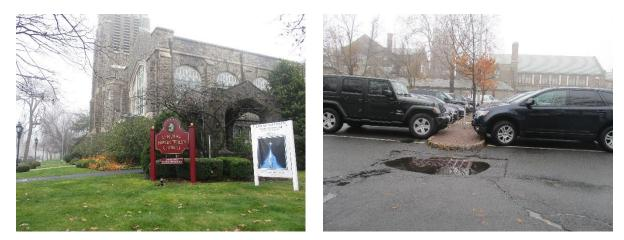
Parking spaces can be replaced with pervious pavement to infiltrate stormwater. A preliminary soil assessment suggests that more soil testing would be required before determining the soil's suitability for green infrastructure.
