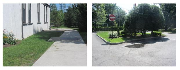
Parking spaces can be replaced with porous asphalt to infiltrate parking lot runoff. A preliminary soil assessment suggests that the soils have suitable drainage characteristics for green infrastructure.
