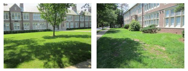
Bioretention systems can be installed around the perimeter of the school to capture, treat, and infiltrate rooftop runoff. A preliminary soil assessment suggests that more soil testing would be required before determining the soil's suitability for green infrastructure.
