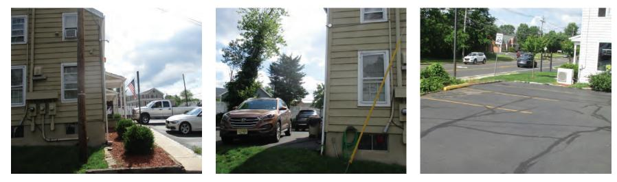
Parking spaces located in the south section of the parking lot can be replaced with pervious pavement to capture and infiltrate stormwater. Downspouts at Annie's Deli can be disconnected and directed into downspout planter boxes to capture and filter rooftop runoff. A preliminary soil assessment suggests that more soil testing would be required before determining the soil's suitability for green infrastructure.
