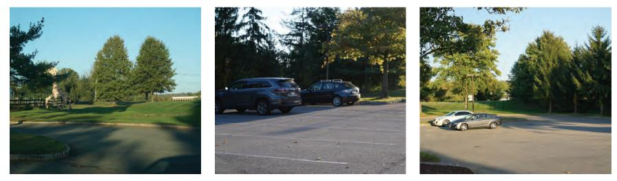
A rain garden can be installed on the eastern island in the parking lot to capture stormwater runoff from the impervious surface. A preliminary soil assessment suggests that more soil testing would be required before determining the soil's suitability for green infrastructure.
