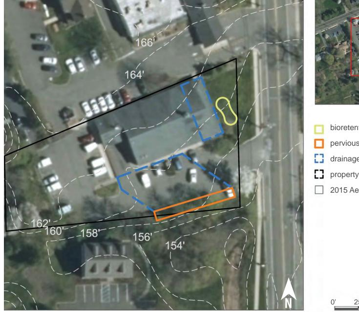
bioretention system pervious pavement drainage area property line 2015 Aerial: NJOIT, OGIS
