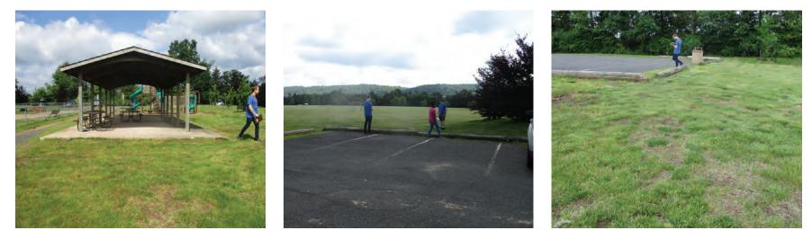
Bioretention systems can be installed to capture, treat, and infiltrate parking lot and rooftop runoff. Potential locations are in the northeast corner of the parking lot and the easternmost side of the structure shown in the above right image. Pervious pavement can be installed in the southwest corner of the parking lot to manage pavement runoff. A preliminary soil assessment suggests that more soil testing would be required before determining the soil's suitability for green infrastructure.
