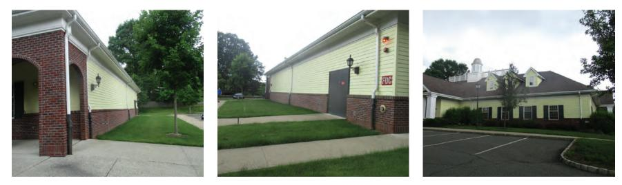
Bioretention systems can be installed to capture, treat, and infiltrate rooftop runoff on the north and south of the building. Pervious pavement can be installed in the southeast corner of the parking lot to capture and infiltrate stormwater. A preliminary soil assessment suggests that the soils have suitable drainage characteristics for green infrastructure.
