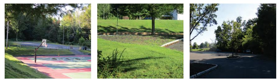
Two sections of parking spaces can be converted to pervious pavement to capture and infiltrate parking lot runoff. Sections of turfgrass adjacent to the parking lot can be converted to rain gardens to capture, treat, and infiltrate parking lot runoff. A preliminary soil assessment suggests that more soil testing would be required before determining the soil's suitability for green infrastructure.
