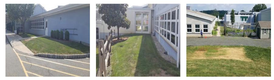
Rain gardens can be installed in the turfgrass to capture, treat, and infiltrate rooftop and parking lot runoff. Downspout planter boxes can be installed in the courtyard to capture and filter stormwater. A preliminary soil assessment suggests that more soil testing would be required before determining the soil's suitability for green infrastructure.
