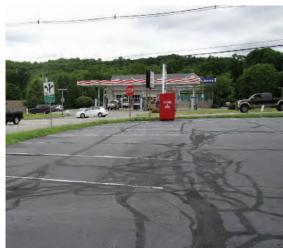
Areas of the parking lot can be retrofitted with porous pavement to capture stormwater runoff from the parking lot. A preliminary soil assessment suggests that the soils have suitable drainage characteristics for green infrastructure.
