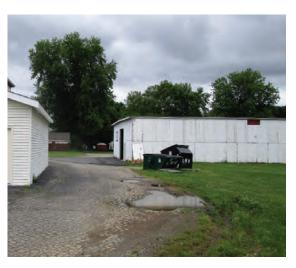
Porous pavement can be installed along the parking spots in the back lot of the building. The downspouts currently empty onto asphalt which is impervious and does not aid in infiltration. A preliminary soil assessment suggests that the soils have suitable drainage characteristics for green infrastructure.
