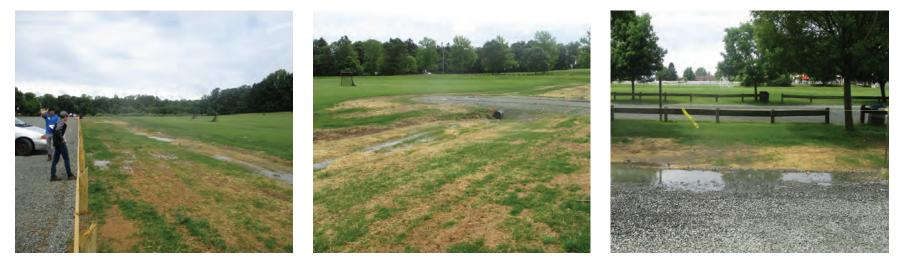
A rain garden can be installed along the northern edge of the parking lot area to help infiltrate the pooling stormwater in that area. A preliminary soil assessment suggests that the soils have suitable drainage characteristics for green infrastructure.
