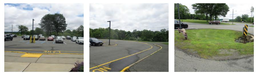
Pervious pavement can be installed in the southernmost row of the parking lot to capture, treat, and infiltrate stormwater runoff from the parking lot. A preliminary soil assessment suggests that the soils have suitable drainage characteristics for green infrastructure
