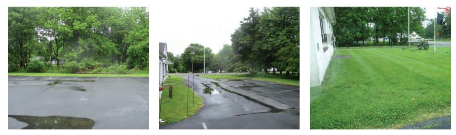
A rain garden can be installed to capture stormwater from the building's rooftop. Pervious pavement can be installed along the northwestern edge of the parking lot to capture the stormwater runoff from the parking lot. A preliminary soil assessment suggests that more soil testing would be required before determining the soil's suitability for green infrastructure.
