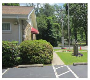
A rain garden can be installed on either side of the entrance to capture stormwater from the rooftop by redirecting the downspout under the sidewalk. Pervious pavement can replace sections of parking spaces to capture a large portion of the parking lot runoff. A preliminary soil assessment suggests that more soil testing would be required before determining the soil's suitability for green infrastructure.
