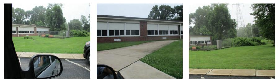
A rain garden can be installed near the disconnected downspouts to capture, treat, and infiltrate rooftop runoff. A preliminary soil assessment suggests that more soil testing would be required before determining the soil's suitability for green infrastructure.
