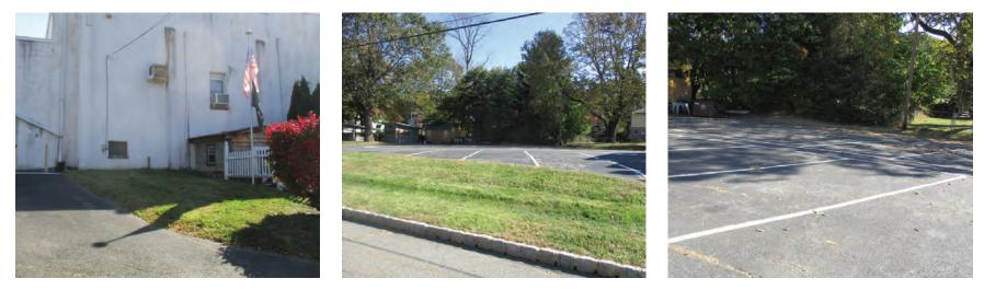
Half of the building's rooftop runoff and part of the parking lot runoff, can be treated with pervious pavement in the east strip of the parking lot. A preliminary soil assessment suggests that more soil testing would be required before determining the soil's suitability for green infrastructure.
