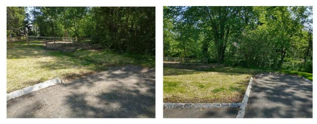
A rain garden can be installed at the beginning of the existing drainage channel to promote infiltration. To prevent standing water and further erosion of the drainage channel, the channel can be converted to a bioswale. A preliminary soil assessment suggests that the soils have suitable drainage characteristics for green infrastructure.
