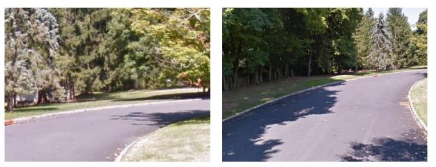
A bioswale can be installed on the corner turn of South Field Drive. This will help with water conveyance down the hill and help prevent erosion alongside the roadway. A preliminary soil assessment suggests that more soil testing would be required before determining the soil's suitability for green infrastructure.
