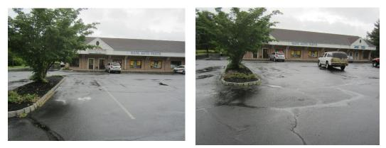
Pervious pavement can be installed at parking spaces adjacent to the building to capture and infiltrate runoff from the parking lot. A preliminary soil assessment suggests that the soils have suitable drainage characteristics for green infrastructure.
