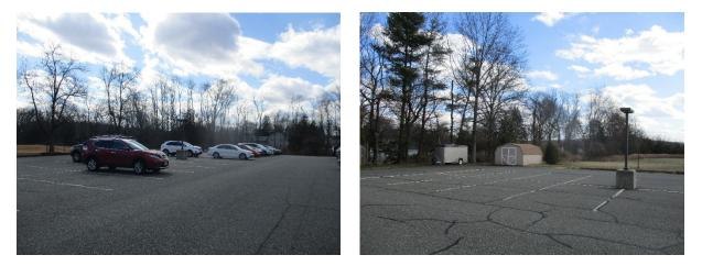
A small strip of turfgrass can be converted to a rain garden to capture, treat, and infiltrate the runoff from the parking lot. A cistern can also be placed adjacent to the building to capture runoff and be used for non-potable purposes such as watering plants. A preliminary soil assessment suggests that more soil testing would be required before determining the soil's suitability for green infrastructure.
