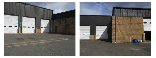
Cisterns can be installed at multiple locations on the buildings to capture stormwater runoff from the roof. This water can be used to wash vehicles or for other non-potable uses. A preliminary soil assessment suggests that more soil testing would be required before determining the soil's suitability for green infrastructure.
