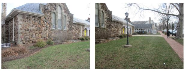
A rain garden can be planted in the patch of turf grass in front of the west entrance to the building. A section of parking spaces can be converted to porous pavement to capture and infiltrate stormwater runoff from the parking lot. A preliminary soil assessment suggests that more soil testing would be required before determining the soil's suitability for green infrastructure.
