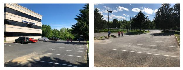
Pervious pavement can be installed in the southern parking lot to help remediate the pooling that occurs due to the pitch of the pavement. Bioretention systems can be installed west of the parking lot to allow for the capture of the parking lot runoff. A preliminary soil assessment suggests that the soils have suitable drainage characteristics for green infrastructure.
