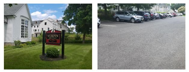
The turfgrass to the southeast of the building can be converted to a bioretention system to help capture, treat, and infiltrate stormwater runoff from the building's roof. Parking spaces in the western portion of the parking lot can be converted to pervious pavement to capture and infiltrate stormwater runoff from the lot. A preliminary soil assessment suggests that more soil testing would be required before determining the soil's suitability for green infrastructure.
