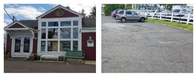
Parking spaces in the parking lot to the north of the building can be converted to porous pavement to capture and infiltrate stormwater runoff from the parking lot. On the north side of the building downspout planter boxes can be installed to help capture stormwater runoff from the building's roof. A preliminary soil assessment suggests that more soil testing would be required before determining the soil's suitability for green infrastructure.
