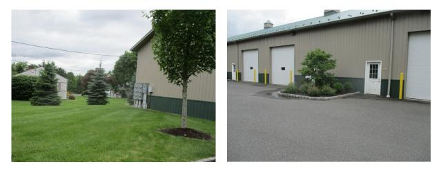
A turfgrass area near the building's southeast corner can be converted to a bioretention system to capture, treat, and infiltrate stormwater runoff from the building's roof. Pervious pavement can be installed between the two buildings, and planter boxes can be installed on the northern side of the east building. A preliminary soil assessment suggests that more soil testing would be required before determining the soil's suitability for green infrastructure.
