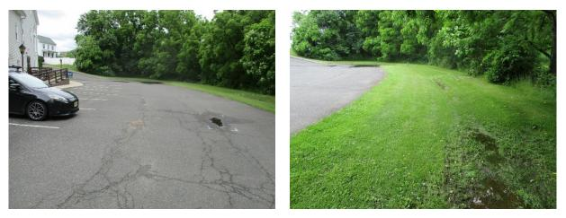
Parking spots on the north side of the building can be converted to pervious pavement to capture and infiltrate stormwater runoff from the building's roof. A bioretention system can be installed at the edge of the parking lot to capture, filter, and infiltrate additional stormwater runoff from the parking lot. A preliminary soil assessment suggests that more soil testing would be required before determining the soil's suitability for green infrastructure.
