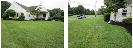
Two bioretention systems are proposed to infiltrate the water from the sloped lawn and a disconnected downspout. A preliminary soil assessment suggests that more soil testing would be required before determining the soil's suitability for green infrastructure.
