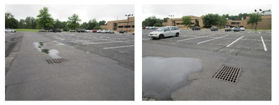
Two mowed detention basins at the east entrance can be retrofitted with rain gardens to capture, treat, and infiltrate stormwater runoff from the driveway and enhance pollinator habitat. Two sections of parking spaces can be converted to porous pavement to capture and infiltrate runoff from the parking lot. A preliminary soil assessment suggests that more soil testing would be required before determining the soil's suitability for green infrastructure.
