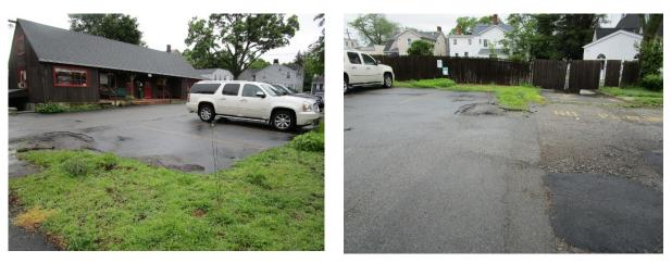
Pervious pavement can be installed to decrease the pooling and erosion caused by the pitch of the pavement and the downspouts leading to the northeast corner of the parking lot. Downspout planter boxes can also be installed to capture runoff from the rooftop. A preliminary soil assessment suggests that the soils have suitable drainage characteristics for green infrastructure.
