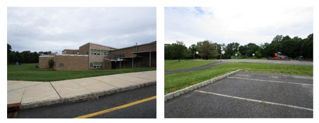
A bioretention system can be installed to the south of the building near the playground to capture, treat, and infiltrate rooftop runoff. A second rain garden can be installed in the low area at the end of the parking lot to better manage the stormwater runoff generated by the parking lot. A preliminary soil assessment suggests that more soil testing would be required before determining the soil's suitability for green infrastructure.
