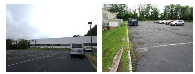
Pervious pavement can be installed in both parking lots to capture and infiltrate stormwater runoff from the parking lot. Bioretention systems can be installed in the turfgrass areas by using curb cuts to direct water from the pavement into them. A preliminary soil assessment suggests that more soil testing would be required before determining the soil's suitability for green infrastructure.
