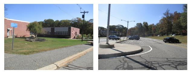
A bioretention system can be created at the south end the building to capture, treat, and infiltrate the building's stormwater runoff. Pervious pavement can be installed in a strip of parking spaces to treat runoff from the parking lot. A preliminary soil assessment suggests that more soil testing would be required before determining the soil's suitability for green infrastructure.
