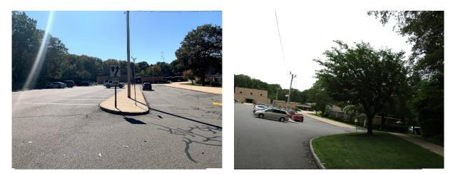
Pervious pavement can be installed in the center parking spaces to capture and infiltrate stormwater runoff from the parking lot. A stormwater planter can be installed by depaving a portion of the wide sidewalk. A curb cut can be used to intercept stormwater runoff from the parking lot. A preliminary soil assessment suggests that the soils have suitable drainage characteristics for green infrastructure.
