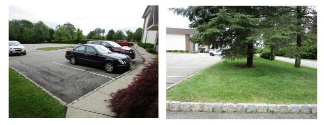
Pervious pavement can be installed on a strip of parking spaces north of the building near connected downspouts. Parking spaces can be replaced with pervious pavement to capture and infiltrate stormwater. The downspouts can be disconnected and redirected into the pervious pavement to capture additional stormwater. A preliminary soil assessment suggests that the soils have suitable drainage characteristics for green infrastructure.
