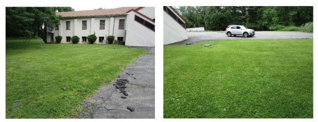
Parking spaces in the parking lot to the southwest of the building can be converted to pervious pavement to capture and infiltrate stormwater runoff from the parking lot. A rain garden can be installed in the turfgrass area west of the building to capture, treat, and infiltrate stormwater runoff from the roof. A preliminary soil assessment suggests that the soils have suitable drainage characteristics for green infrastructure.
