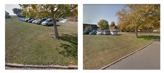
A rain garden can be installed in the north of the eastern parking lot to capture, treat, and infiltrate stormwater runoff from the parking lot before reaching the nearby storm drain. A preliminary soil assessment suggests that the soils have suitable drainage characteristics for green infrastructure.
