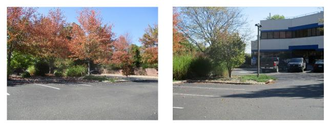
Parking spaces west of the building can be converted to pervious pavement to capture and infiltrate stormwater runoff from the road and parking lot. A preliminary soil assessment suggests that more soil testing would be required before determining the soil's suitability for green infrastructure.
