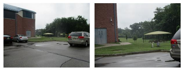
A rain garden can be installed south of the gym building to capture, treat, and infiltrate stormwater runoff from the roof. The nearby downspouts can be disconnected into the rain garden. Parking spaces west of the gym can be converted to porous pavement to capture and infiltrate stormwater runoff from the parking lot. A preliminary soil assessment suggests that more soil testing would be required before determining the soil's suitability for green infrastructure.
