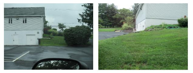
A rain garden can be installed south of the building to capture, treat, and infiltrate rooftop stormwater runoff. A preliminary soil assessment suggests that the soils have suitable drainage characteristics for green infrastructure.
