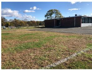
A rain garden can be installed adjacent to the northeast corner of the parking lot to capture, treat, and infiltrate runoff from the parking lot. Additionally, two raingardens can be installed to treat the rooftops of the adjacent buildings. A preliminary soil assessment suggests that the soils have suitable drainage characteristics for green infrastructure.
