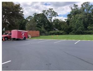
Parking spaces can be converted to porous pavement to capture and infiltrate stormwater runoff from the parking lot. A rain garden can be installed in the turfgrass area near the entrance of the building to capture, treat, and infiltrate stormwater runoff from the roof. A preliminary soil assessment suggests that more soil testing would be required before determining the soil's suitability for green infrastructure.
