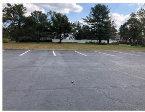
Parking spaces in the parking lot to the east of the building can be converted to porous pavement to capture and infiltrate stormwater runoff from the parking lot. Rain gardens can be installed in the turfgrass at the entrance and rear of the building to capture, treat, and infiltrate stormwater runoff from the roof. A preliminary soil assessment suggests that more soil testing would be required before determining the soil's suitability for green infrastructure.
