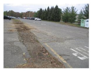
A row of parking spaces to the north of the main building can be converted to porous pavement to capture and infiltrate stormwater runoff from the parking lot and roof. Rain gardens can be installed at various locations to capture, treat, and infiltrate stormwater runoff from the roof. A preliminary soil assessment suggests that the soils have suitable drainage characteristics for green infrastructure.
