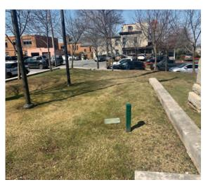
The runoff from the stairway can be intercepted prior to reaching the street by installing a hybrid system of a tree filter box and a stormwater planter. A preliminary soil assessment suggests that more soil testing would be required before determining the soil's suitability for green infrastructure.
