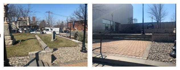
The runoff from the stairway can be intercepted prior to reaching the street by installing a hybrid system of a tree filter box and a stormwater planter. A preliminary soil assessment suggests that more soil testing would be required before determining the soil's suitability for green infrastructure.
