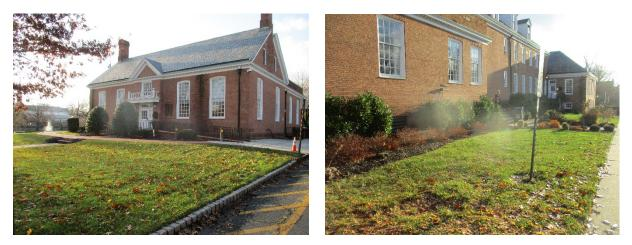
Five rain gardens can be installed in the turfgrass areas around the building to capture, treat, and infiltrate stormwater runoff from the roof of the building.
