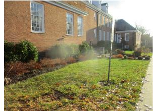
Five rain gardens can be installed in the turfgrass areas around the building to capture, treat, and infiltrate stormwater runoff from the roof of the building. A preliminary soil assessment suggests that more soil testing would be required before determining the soil's suitability for green infrastructure.
