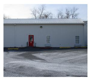
Parking spaces near the firehouse can be converted to pervious asphalt to capture and infiltrate runoff from the rest of the parking lot and from the roof of the eastern building. Downspouts on the western building can be redirected to a cistern to collect rainwater for non-potable uses, such as for washing firetrucks. A preliminary soil assessment suggests that more soil testing would be required before determining the soil's suitability for green infrastructure.
