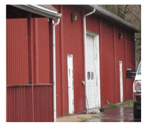
A rain garden can be installed in the turfgrass area on the west side of the building to capture, treat, and infiltrate stormwater runoff from the roof. The downspout at the southeast corner of the building can be connected to a downspout planter box to allow rooftop runoff to be filtered and reused. A preliminary soil assessment suggests that more soil testing would be required before determining the soil's suitability for green infrastructure.
