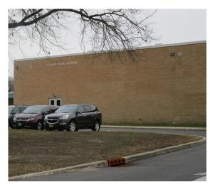
The two parking lots on both the east and west sides of the school can be converted to porous pavement to treat the stormwater runoff from the roof of the elementary school. A preliminary soil assessment suggests that more soil testing would be required before determining the soil's suitability for green infrastructure.
