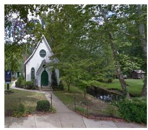
Parking spaces in the parking lot behind the church building to the northwest can be converted to pervious pavement to capture and infiltrate stormwater runoff from the parking lot and roof of the church. A rain garden can also be installed at the front of the church and downspouts can be directed under the sidewalk into the large turfgrass area. A preliminary soil assessment suggests that more soil testing would be required before determining the soil's suitability for green infrastructure.
