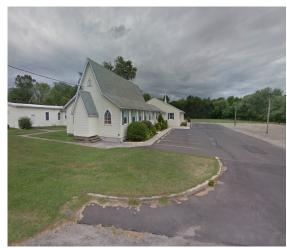
Two rain gardens can be installed in the turfgrass area near the entrance of the building to capture, treat, and infiltrate stormwater runoff from the roof. The garden will also add aesthetic value to the surrounding area. A preliminary soil assessment suggests that more soil testing would be required before determining the soil's suitability for green infrastructure.
