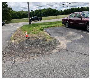
A rain garden can be installed in the turfgrass area near the roadway. The rain garden will collect runoff from the parking lot via curb cuts and regrading the lot. Two additional rain gardens can be installed on each side of the entrance by directing downspouts to capture runoff from the rooftop. A preliminary soil assessment suggests that the soils have suitable drainage characteristics for green infrastructure.
