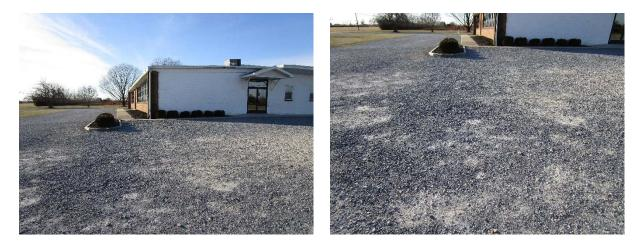
Parking spaces east of the church can be replaced with pervious pavement to capture and infiltrate stormwater runoff from the lot and rooftop runoff from the church. A preliminary soil assessment suggests that more soil testing would be required before determining the soil's suitability for green infrastructure.
