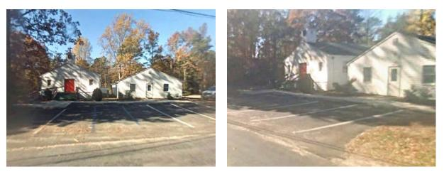
Parking spaces southeast of the church can be replaced with pervious pavement to capture and infiltrate stormwater from surrounding parking spaces and from the nearby street. A preliminary soil assessment suggests that the soils have suitable drainage characteristics for green infrastructure.
