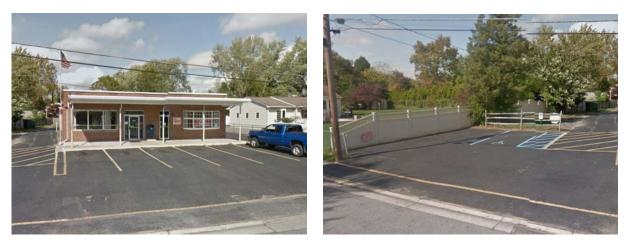
Parking spaces southwest and southeast of the post office can be replaced with pervious pavement to capture and infiltrate stormwater from the parking lot and rooftop runoff from the building. A preliminary soil assessment suggests that the soils have suitable drainage characteristics for green infrastructure.
