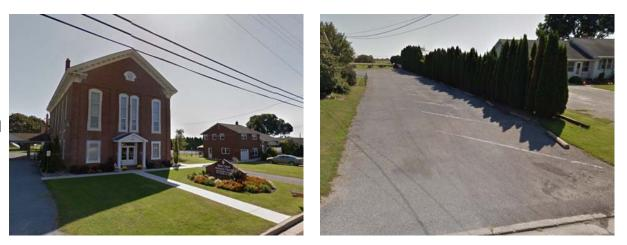
Parking spaces surrounding the church can be replaced with pervious pavement to capture and infiltrate stormwater runoff from the street and from the remainder of the parking lot. A preliminary soil assessment suggests that more soil testing would be required before determining the soil's suitability for green infrastructure.
