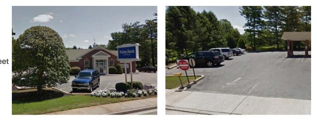
Parking spaces east and west of the bank can be replaced with pervious pavement to capture and infiltrate stormwater runoff from the remainder of the parking lot and rooftop runoff from the bank. A preliminary soil assessment suggests that more soil testing would be required before determining the soil's suitability for green infrastructure.
