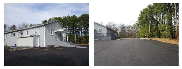
The southern half of parking spaces northeast of the building can be replaced with pervious pavement to capture and infiltrate stormwater. A preliminary soil assessment suggests that the soils have suitable drainage characteristics for green infrastructure.
