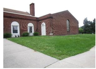
Bioretention systems can be installed in the turfgrass areas in the front of the building. Bioretention systems can capture, treat, and infiltrate rooftop runoff. A preliminary soil assessment suggests that more soil testing would be required before determining the soil's suitability for green infrastructure.
