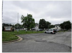
Parking spots at the entrance of the building can be replaced with pervious pavement which will capture and infiltrate stormwater from the parking lot. A bioretention system can be installed at the front of the building to capture runoff from the rooftop. A preliminary soil assessment suggests that more soil testing would be required before determining the soil's suitability for green infrastructure.
