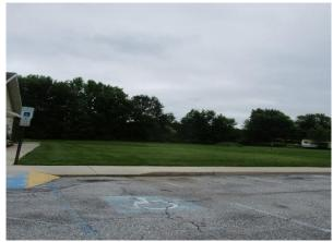
On the north and south side of the building, a bioretention system can be installed in the turfgrass area. Bioretention systems can be installed to capture, treat, and infiltrate rooftop runoff. Bioretention systems add aesthetic value to a location while also managing stormwater. A preliminary soil assessment suggests that more soil testing would be required before determining the soil's suitability for green infrastructure.
