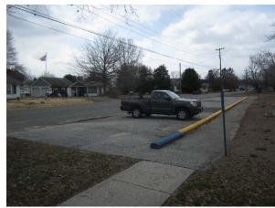
A bioretention system can be installed at the southwest corner of the building by redirecting downspouts to capture rooftop runoff. A strip of parking spaces to the west side of the building can be replaced with pervious pavement to capture and infiltrate stormwater. A preliminary soil assessment suggests that the soils have suitable drainage characteristics for green infrastructure.
