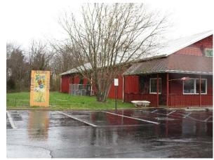
A rain garden can be installed in the turfgrass area on the west side of the building to capture, treat, and infiltrate stormwater runoff from the roof. The downspout at the southeast corner of the building can be connected to a downspout planter box to allow rooftop runoff to be filtered and reused. A preliminary soil assessment suggests that more soil testing would be required before determining the soil's suitability for green infrastructure.
