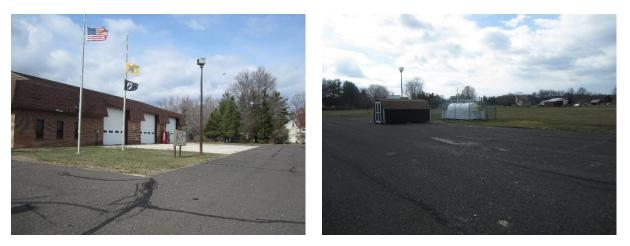
A bioretention system can be installed in the turfgrass area behind the sign and in front of the flag poles to allow stormwater runoff from the parking lot to infiltrate through the soil. Sections of the parking spaces can be converted to pervious pavement to allow water from the pavement to infiltrate into the ground. A preliminary soil assessment suggests that the soils have suitable drainage characteristics for green infrastructure.
