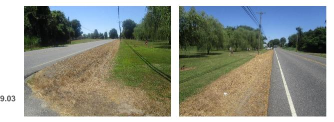
The trench stretching along the east side of the road can be converted into a rain garden to allow stormwater runoff from the road to infiltrate more efficiently. Creating a rain garden will also benefit wildlife by creating habitat. A preliminary soil assessment suggests that more soil testing would be required before determining the soil's suitability for green infrastructure.
