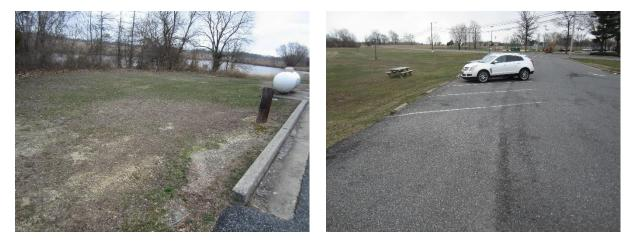
Bioretention systems can be installed in turfgrass at two locations to allow the stomrwater runoff from the pavement to infiltrate. The parking spaces east of the pizzeria can be retrofitted with pervious pavement to allow water to penetrate the surface. A preliminary soil assessment suggests that more soil testing would be required before determining the soil's suitability for green infrastructure.
