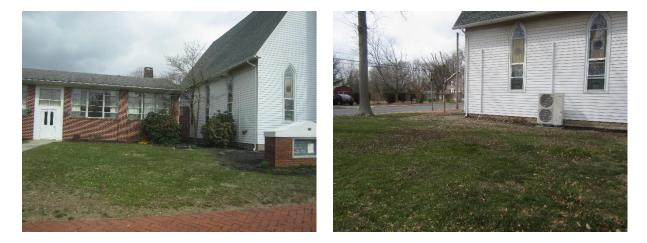
A bioretention system can be installed in the turfgrass area near the entrance of the building by the sign as well as the turfgrass area at the southeast side of the building to capture, treat, and infiltrate stormwater runoff from the roof. A preliminary soil assessment suggests that more soil testing would be required before determining the soil's suitability for green infrastructure.
