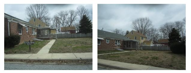
Bioretention systems can be installed in the turfgrass on both sides of building to capture, treat, and infiltrate stormwater runoff from the roof. A preliminary soil assessment suggests that more soil testing would be required before determining the soil's suitability for green infrastructure.
