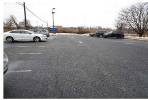
A section of parking spaces can be converted to porous pavement to capture and infiltrate stormwater runoff from the parking lot and part of the roof. A preliminary soil assessment suggests that more soil testing would be required before determining the soil's suitability for green infrastructure.
