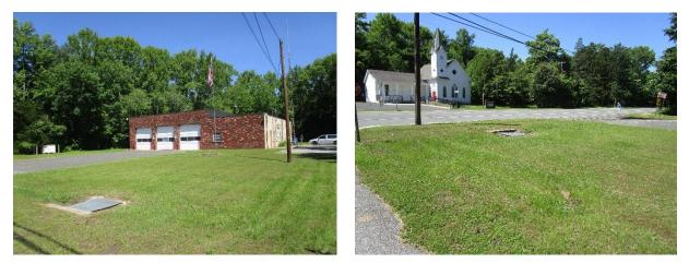
A rain garden can be installed in the turfgrass close to the road to capture, treat, and infiltrate stormwater runoff from the roadway before entering the catch basin. Cisterns can be installed at the downspouts to capture rooftop runoff. The water can then be used to wash cars, water landscaping, or for other non-potable purposes. A preliminary soil assessment suggests that more soil testing would be required before determining the soil's suitability for green infrastructure.
